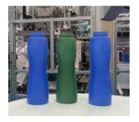
At the JSW booth, we conducted a live demonstration of our flagship blow molding machine, the MBD-C33A/54E2Z-AP(C3). The machine produced 1L three-layer bottles with PCR material in the middle layer, demonstrating our multilayer technology that meets the European market's strong focus on sustainability. We also introduced our enhanced remote
