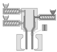
Multi-layer package is produced with co-extrusion direct blow molding machine which has extruders as many as numbers of constructed resins. These resins are layered by flowing along designed resin route and come out from the head as layered parison. Because of this process, direct blow molding is the most suitable machine to produce multi-layer package.
