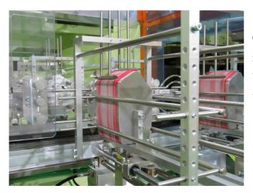
The IML carriage unit picks up the labels from the magazines and inserts them in the molds of a blow molding machine with a high speed.
