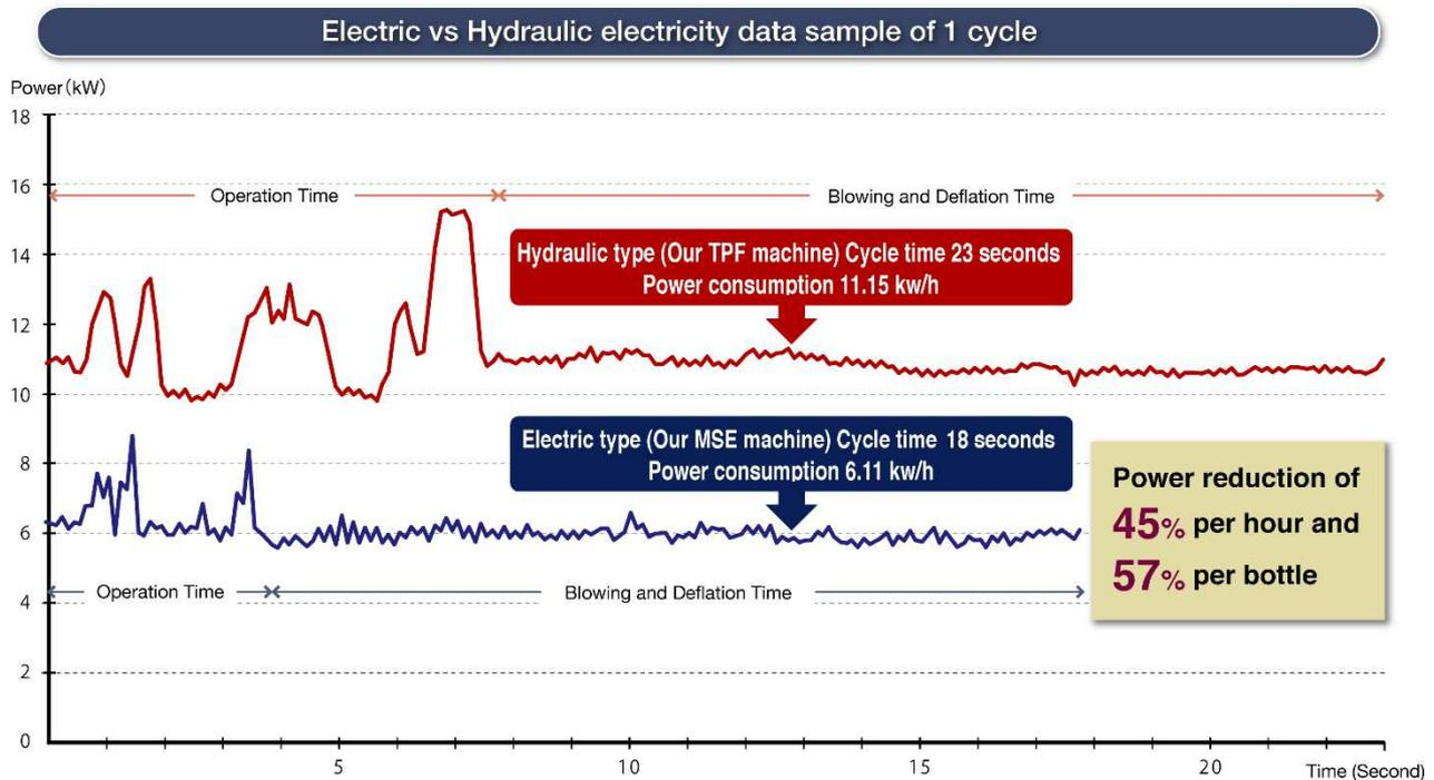
※1 The above data is measured by using 2 parison single station machines to mold same size of single layer PP bottles (500ml, 50g).
